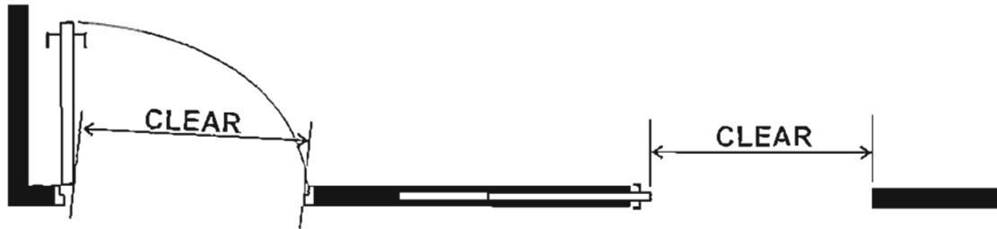
Figure 1. Clear Opening Measurement For Doors
